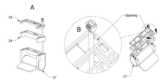
A. Position the White Foot Pedal Cable (36) to exit the stacked Spacers (33-34) on the right- or left-side, based on where you have placed the Engine Box (21) in the sink cabinet. The White Foot Pedal Cable (36) should be directed through the corresponding notch on the side of the Spacer(s) (33-34) stacked on the Foot Pedal (27).
