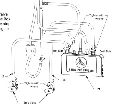
A. Secure the Engine Box (21) onto the Engine Box Wall Mount (22). Center the Engine Box (21) on the Engine Box Wall Mount (22) and press against the wall until you feel the Engine Box (21) slip over the Engine Box Wall Mount (22) and then press down firmly to lock it into place.
