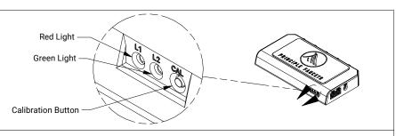
3. Wait until the lights have changed to the following pattern: Red Light (<u>blink once with a pause</u>) and Green Light (<u>solid</u>). While the Foot Pedal (27) is in the up/rest position, press and release the CAL button once.
