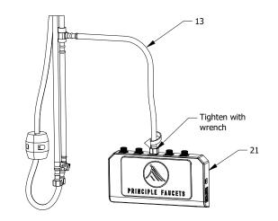
A. Connect the Faucet Supply Hose - Cold/Blue (14) and Faucet Supply Hose - Hot/Red (15), located at the base of the Faucet Body (1), to the cold output (center right) and hot output (center left) connections on the Engine Box (21). Tighten firmly with a wrench.
